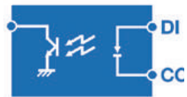
2500Vrms Opto-isolation Digital Input
