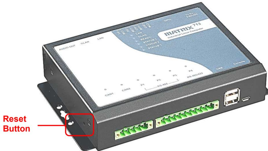
The behavior of the reset button depends on how long you press the reset button.
