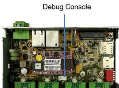
Pin assignment is: RX, TX, +3.3V, GND.
