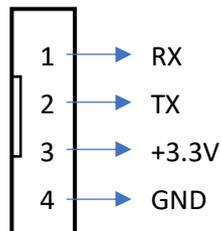
Therefore, you need to open the upper metal case and prepare or purchase a serial console cable to use the serial console port.
