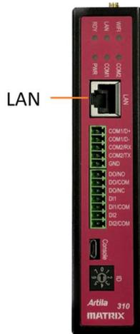
The Ethernet Port use RJ45 connector. Pin-Assignment as below:
